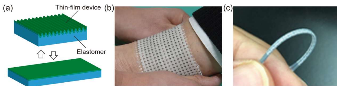
Figure 1. (a) Film/elastomer structure. (b) Kirigami-structure device. (c) Fiber-shape device
