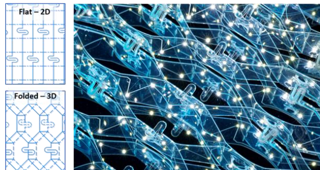
Figure 1. Close-up photograph of a folded LED lighting foil with a hexagonal structure.
